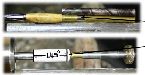
How the parts fit showing the tube placements. Notice the tubes do not meet.
