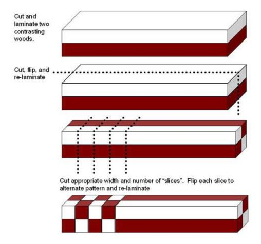
Tips - Good, square, 90 degree cuts are a must. Your pattern also must be well centered. What I mean is, the hole you drill down the length of the laminated pen blank must be as centered as possible. If off set or not centered, you will have smaller checker squares on one side of the pen and larger on the other.
