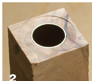
2 Square the blank before turning.
