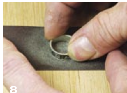
For a seamless transition, square the ring on a piece of sandpaper.
