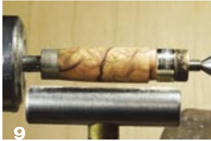
9 With a skew, turn a gentle curve.
