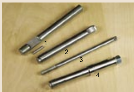
Fixtures for turning closed-end pens: pin chuck (1), home-made expansion chuck (2), tap mandrel (3), and commercial expansion chuck (4).
