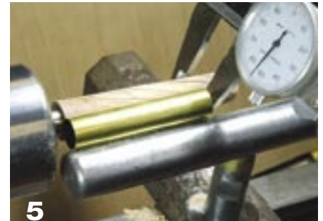
Measure the thickness at the end of the internal brass tube to avoid breaking through on the blank.
