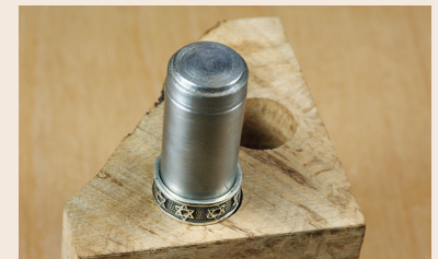
A conical steel round will allow you to slightly expand a sterling-silver ring.
