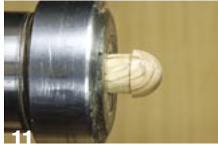
11 Chuck the tube and turn the finial to shape.
