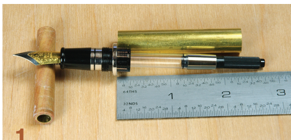
1 To determine the drill depth, assemble the pump on the front section.
