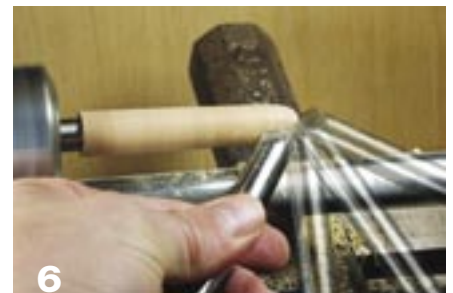
Using a diamond-point tool is an easy way to round over the end of the main body.
