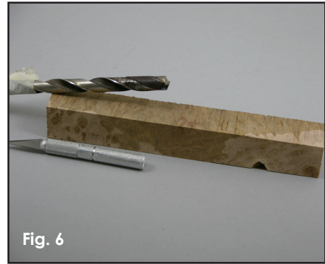
A little tape on the bit acts as a depth gauge.
