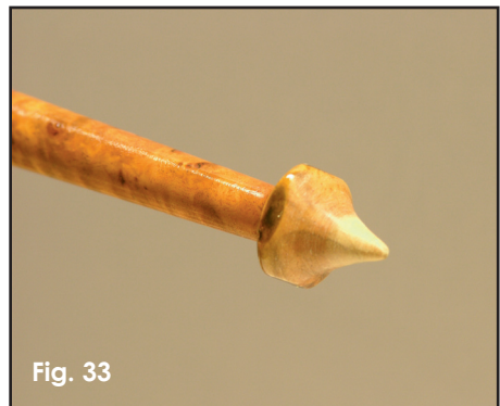
Be sure to support the fragile end with your fingers until it is parted free.
