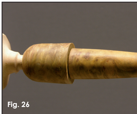
A slight uniform gap indicates that the tapers are mating properly.
