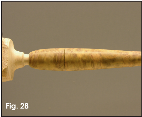
Turn the excess material from the nosepiece.
