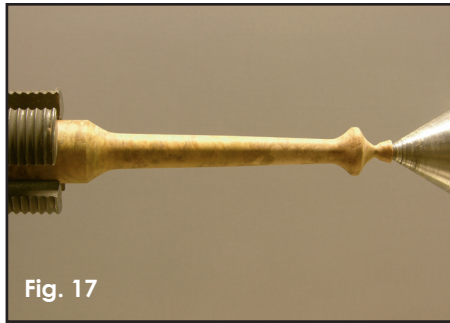
Fig. 17 Get as close to the final shape as possible.
