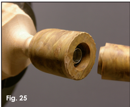
Cut the mating angle on the nosepiece.
