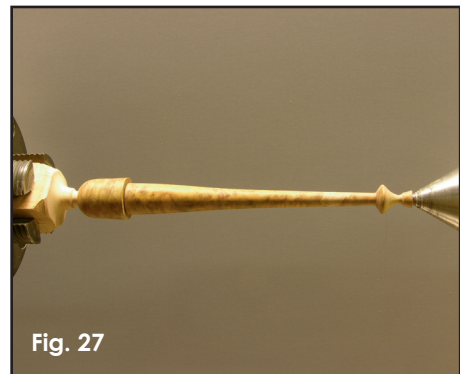
Remount the handle in the lathe along with the nosepiece.
