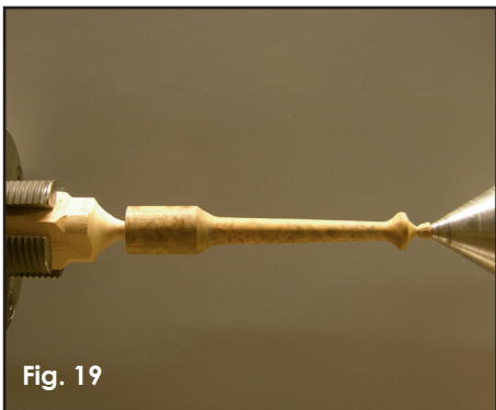
Fig. 19 Bring up the tailstock for additional support.
