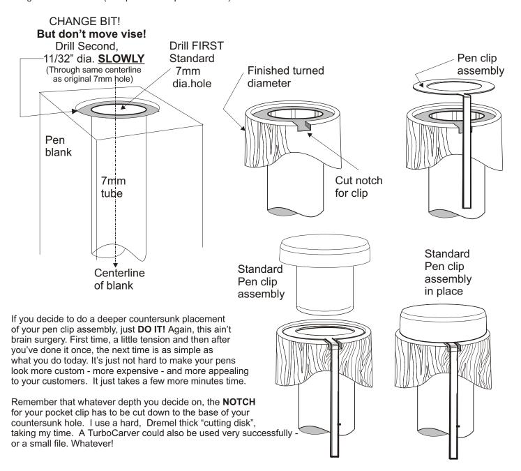
I also use a **black** felt marker and color the cut **edges** I've made for the pocket clip cutout. I also blacken all the interior of the 11/32" hole I've drilled. It just hides any discoloration or imperfection in drilling through different materials, which can leave the normal scratches of a drill or file or cutting disk - the black marker is permanent and waterproof - just makes it all look "finished" - AND more professional.
