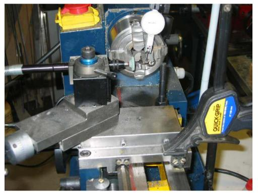
pen mill. The carriage is locked to prevent movement. I don't have a lock (yet) so I used a clamp.
