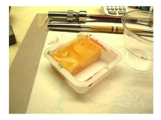
Above shows a block that was molded - then removed, a blank bandsawed away and then the block was re-positioned into the mold, just to show how it first appeared.
