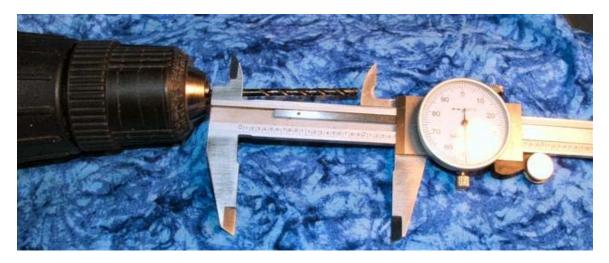
Now drill out nib end until the jaws or face of chuck bottom.
