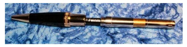
Check final fit and function. Note: you must twist the mechanism and manually return it counterclockwise for this modification to work correctly.
