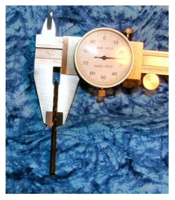
And chuck it into a cordless drill so the point is 2.450" from the jaws or front face of the chuck (this is critical for proper fit)
