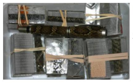
Blanks cut from the castings, standoffs, corks, BBs removed. Paired together and ready to turn. A finished baron is also included.
