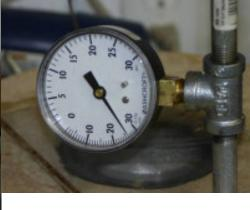
Just for reference, here is a picture of my pump and the gauge which is reading 23 or so inches of Hg. The next picture shows the pressure tank with the homemade lid for using the vacuum set-up.
