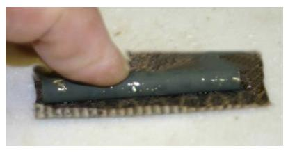
Set the tube on the glue bead and hold until set. Then roll the tube to one side and the glue will squeege in front of it. Turn the tube/skin around and place another bead of glue next to the tube and roll it toward the end. Overlap this second edge over the first edge. Do not try a butt joint. The overlapping joint is the only one to use.
