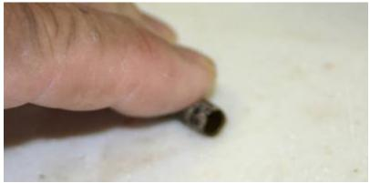
Roll the tube under your fingers to insure the skin is tightly glued to the tube. Pay close attention to the seam and the edges. Apply moderate pressure to press the seam together and the edges against the ends of the tubes.
