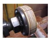
already in the faceplate The faceplate is mounted on the lathe for truing and balancing.
