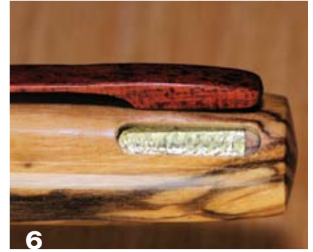
6 The finished pen-clip mortise on the cap is routed to the brass tube. Check the fit with the clip before adhering with epoxy.
