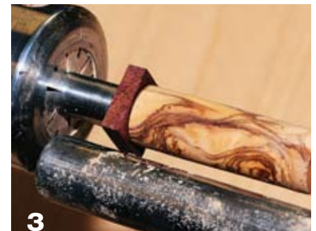
For a centerband, glue a predrilled \frac{1}{4} "-thick piece of wood at the end of the cap. Turn the final dimension to 0.600".
