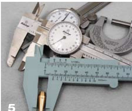
5 Dial calipers will produce consistent measurements for barrel diameters.
