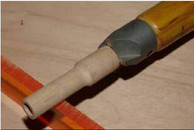
Picture 7: A custom shim for squaring the cap ends
