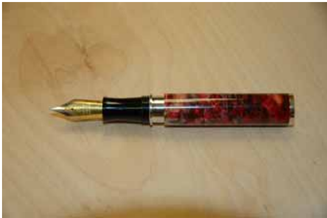
Picture 9: Lining the nib up with the sunny side of the body
