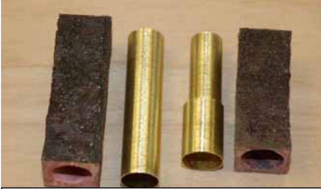
Picture 5: The 3 brass tubes and 2 drilled blanks
