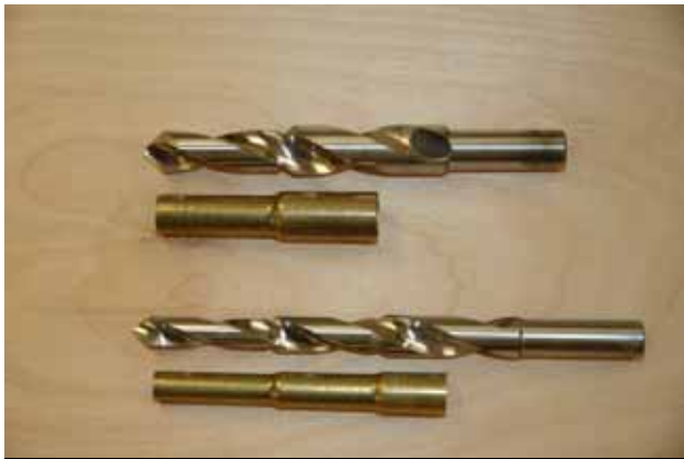
Picture 1: Stepped tubes and dedicated drill bits, from another kit, not used here
