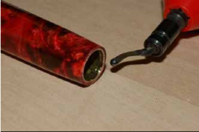
Picture 11: A deburring tool is used to put a little slope on the end of the brass tube
