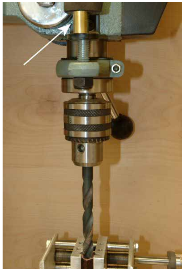
Picture 4: Using the large tube to set the depth stop for the second drill operation for the cap
