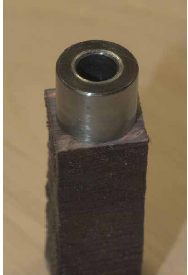
Picture 6: Testing the accuracy of the drilling of this marginal blank
