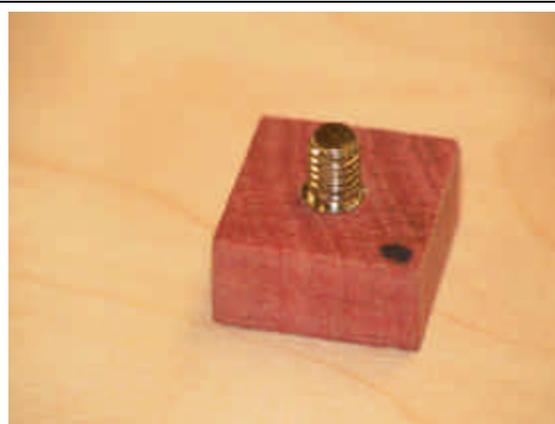
**Fig. 11: The finial blank, ready for turning**
