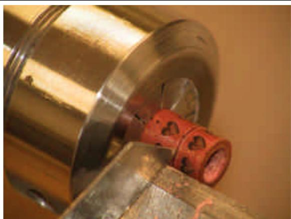
**Fig. 3: Parting off the centerband with the narrow parting tool**
