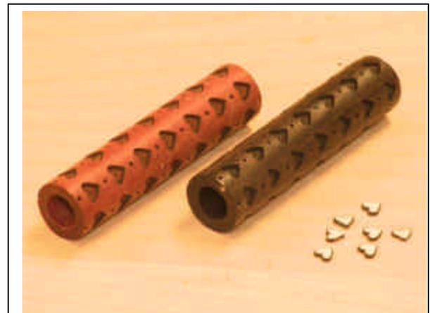
**Fig. 1: These two barrels have just come back from the engraver. They will yield 14 center-bands Also shown are hearts lasercut from ivory to fit the heart pockets perfectly.**
