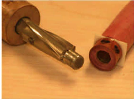
**Fig. 7: The centerband is glued up with an ivory spacer. nother recess has been cut using the piloted counterbore shown**
