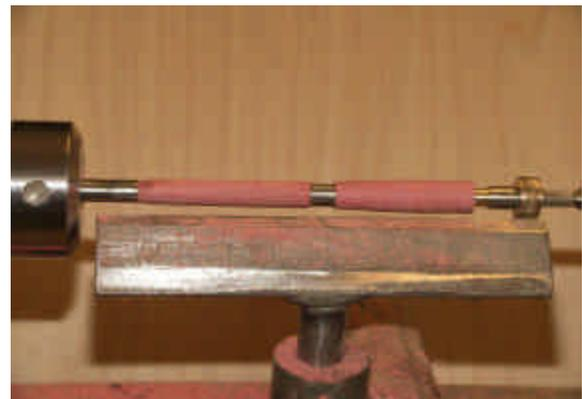
**Fig. 6: These are rough-turned penbarrels. The cap barrel has had a tenon turned to receive the centerband**
