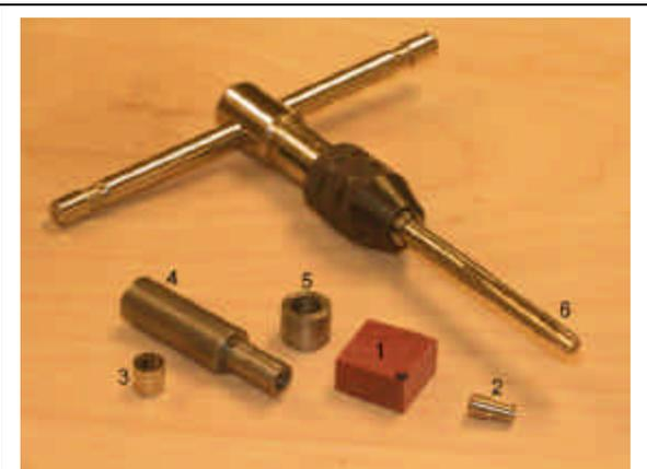
**Fig. 8: The materials and tools used to make a custom finial. (1) wood blank, (2) cap stud, (3) finial adapter fitting, (4) cap stud mandrel, (5) homemade bushing, (6) bottom tap in handle**
