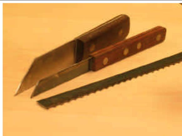
**Fig. 2: A commercial narrow parting tool, a homemade even narrower parting tool, and the saw blade from which it was made**
