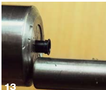
13 Hold the nib housing in a Beall collet chuck and reduce the tenon to 0.336".
