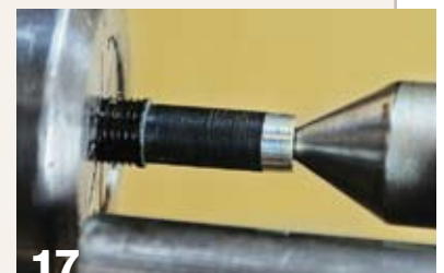
17 Grip the El Grande section in a collet, add the little support disk, and use a live center in the dimple. Turn away the contoured grip to a .335" diameter for a slip-fit Broker tube.
