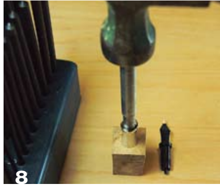
8 To knock out the threads from the grip, use a \frac{19}{64} " punch and block with a 10mm hole.
