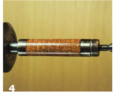
4 With the cap mounted between bushings, turn the stock to a 0.650" diameter.
