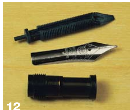
12 Screw the nib housing into the threaded fitting knocked out from the original grip.
