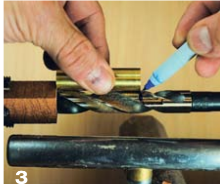
3 Use the cap brass tube to precisely mark the drilling depth.
