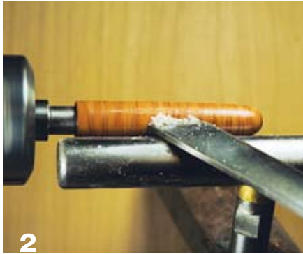
2 With an old skew gently scrape cured cyanoacrylate (CA) from the body.
