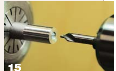
15 A centering drill is ideal for drilling aluminum rod.
