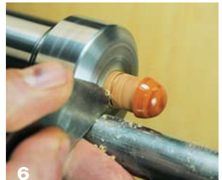
6 Part off the final cap, leaving a \frac{1}{2} "-long tenon.
