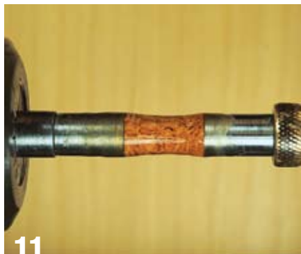
11 Turn the grip between centers and finish with thin CA glue.
